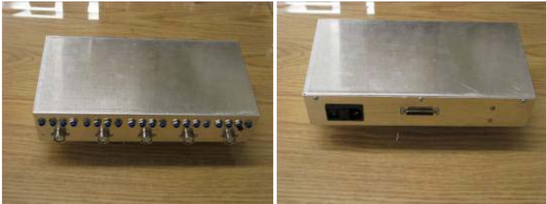
Fig. 3.9: Front and back of the new multi sensor probe circuit box
