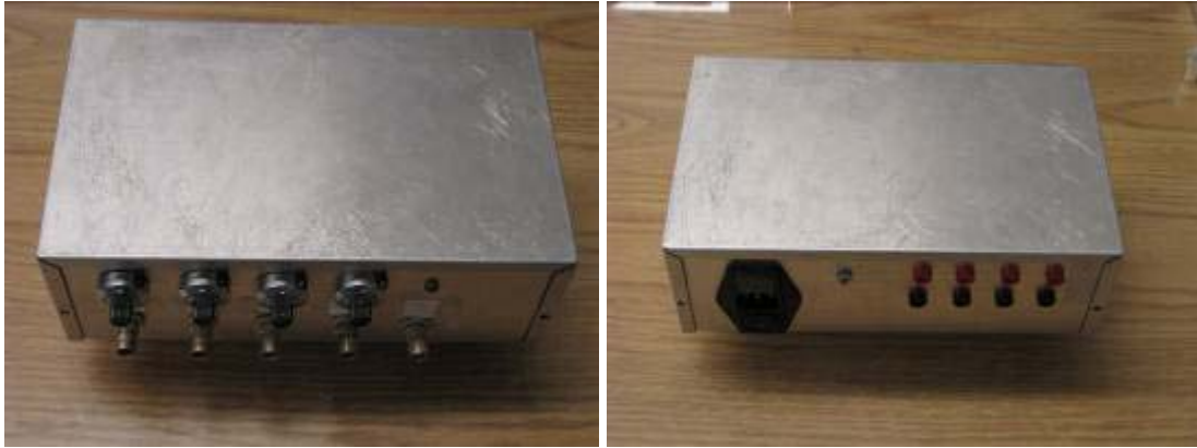
Fig. 3.8: Front and back of a conventional multi sensor probe circuit box.
